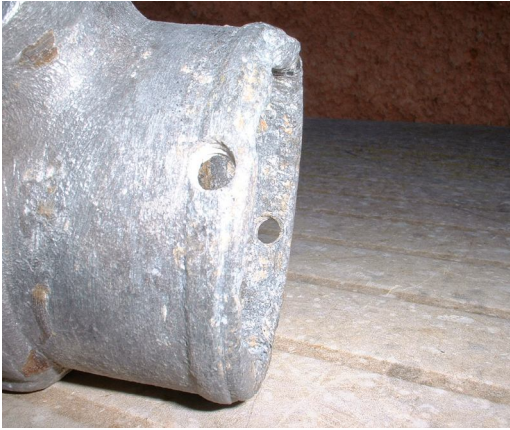
Old epoxy resin cleaned up showing pitting and corrosion. Note resin failed to remain attached.
